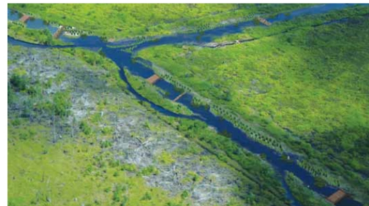
An illustration of the planned hydrological rehabilitation system in KFCP. Compacted peat dams, palisades and reforestation are visible along the canals.
