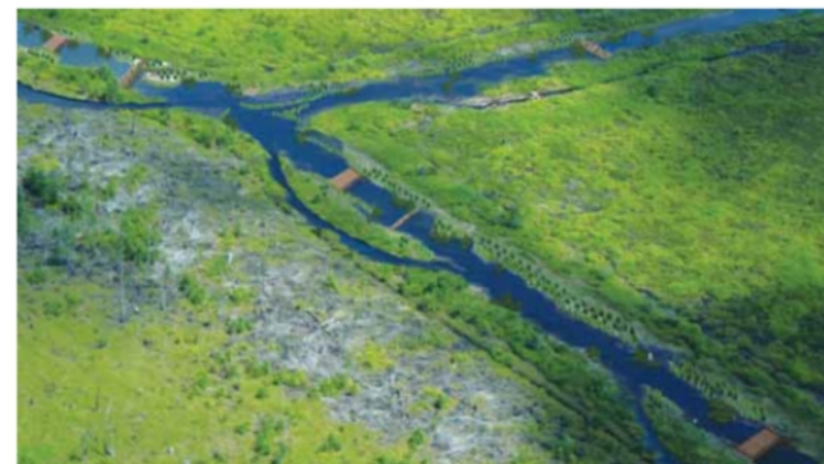
An illustration of the planned hydrological rehabilitation system in KFCP. Compacted peat dams, palisades and reforestation are visible along the canals.
